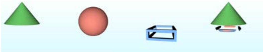
■ Figure 3 Sample image with operations: Cone (Union) + Sphere (Union) + Box Frame (Subtraction)
